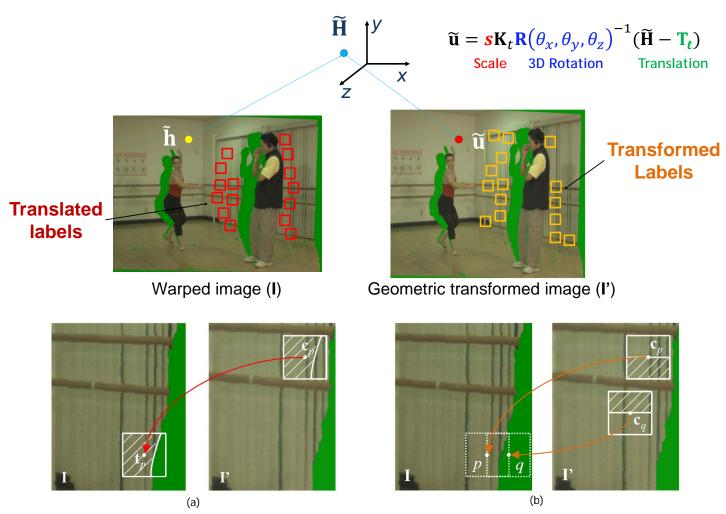
Illustration of the proposed 3D geometric transformation based view synthesis method for wide angle view.
